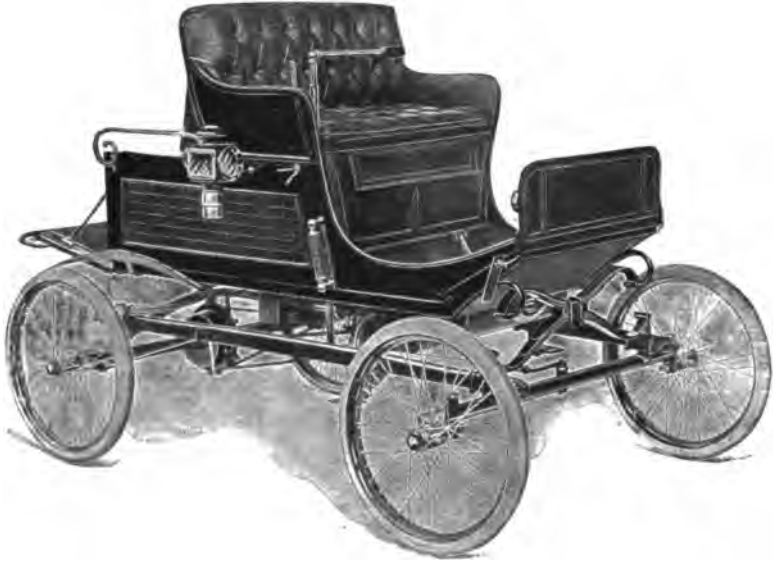
FIG. 74.—One Model of the Stearns Steam Carriage, showing the perch rods of hickory wood, which give a much more flexible frame than steel tubes, without the numerous difficulties involved in the use of swivel joints.
